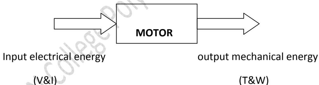
The machine which operates as a generator can also be operated as a motor with same constructional features. when the DC machine converts mechanical energy into electrical energy called as DC generator. Where as the DC machine converts electrical energy into mechanical energy is called a DC motor. This process is called electro mechanical energy conversion process.
