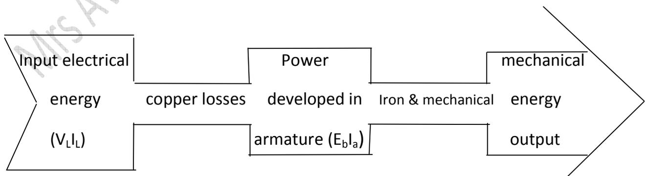
$$\text{Electrical efficiency } (\eta_{\text{ele}}) = \frac{\text{Power developed in armature } (E_b I_a)}{\text{Input electrical energy } (V_L I_L)}$$
