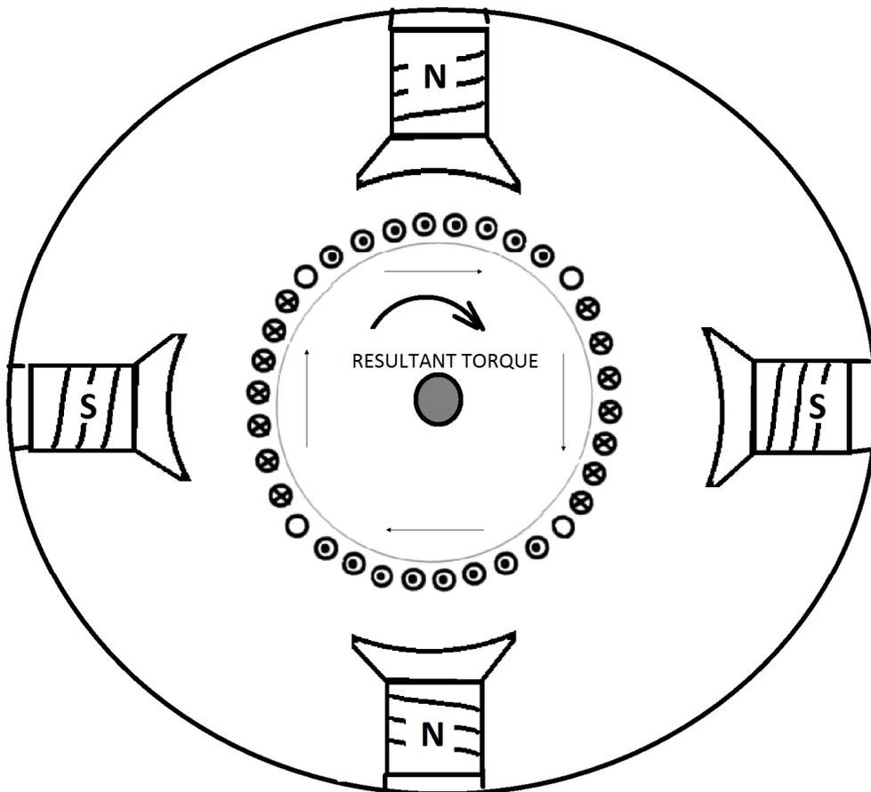
Let us consider a multi polar DC motor as shown in above figure. The field magnets are excited to develop alternate north(N) and south(S) poles and the armature conductors carrying current is placed between magnetic field.
